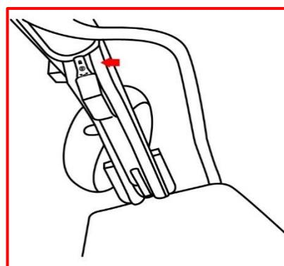
After unfold your scooter, don't forget to put the safety lock
