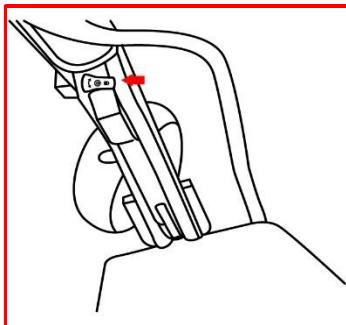
To fold your scooter, remove the safety lock and push to fold the scooter.
