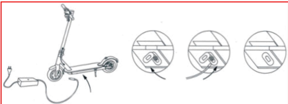
When loading your scooter make sure that the loading port is in good condition and that no residue is trapped inside. If this is the case, clean it with a dry cloth. Use the charger supplied with the product, and only this charger. If you have lost your charger, or if it is faulty, contact the Urbanglide support. Once the charger displays a green light, unplug your product. Do not leave the charger plugged in for too long after charging is complete.
