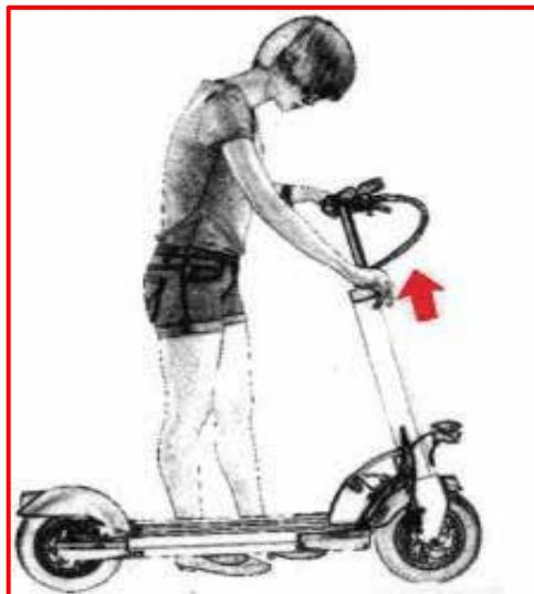
Adjust the size of your handlebars by loosening the clamping buckle located on the stem. Be careful not to exceed the height limit indicated. Check that your handlebars are stable and that the clamp is tight.
