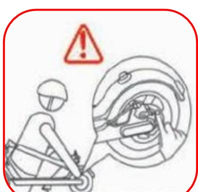
Do not touch the disc brakes after using your scooter, these parts can be hot after a long ride.
