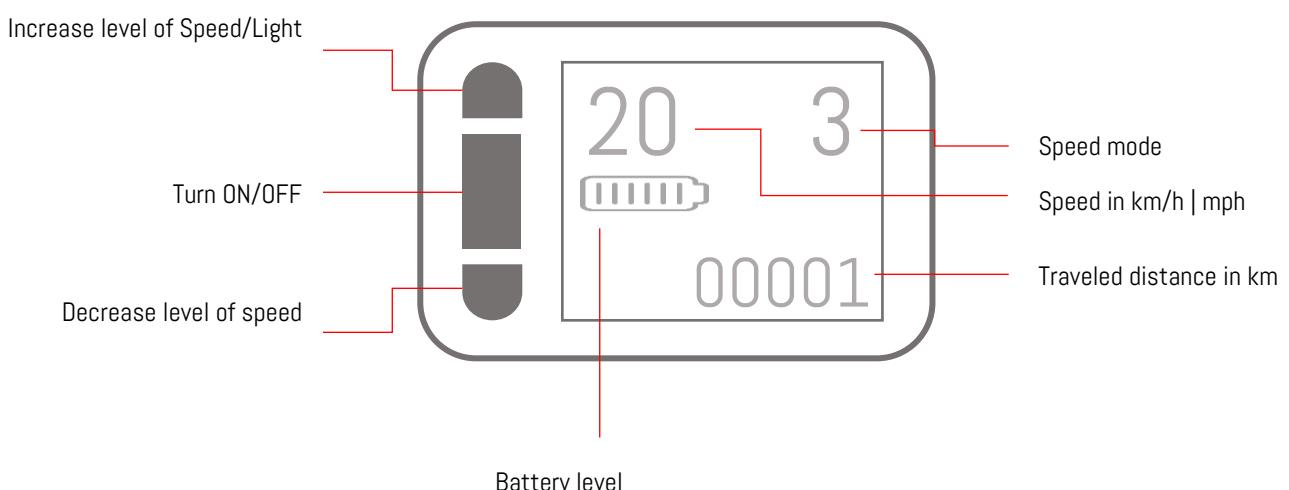
First, turn on your product by pressing the "Power" button on the handlebar. Check that your battery is charged.
