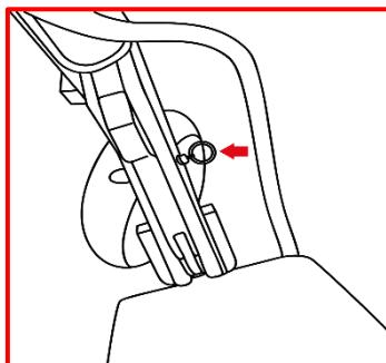
To be able to pull on the folding handle, the safety must be removed by pulling on the loop located on the right.
