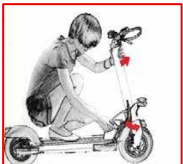
Then return the safety buckle to its original position, and make sure that your handlebars are stable.
