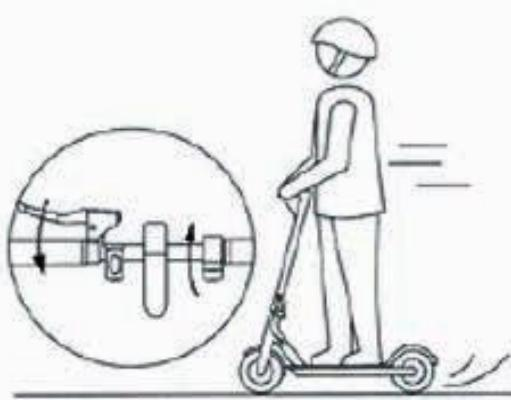
To brake, gently squeeze the brake levers on your handlebars.
