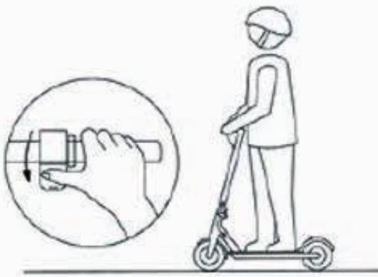
Gently squeeze the throttle trigger to begin picking up speed.
