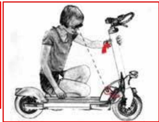
Then pull the folding handle and lower the stem to your scooter deck. Once lowered to the maximum, return the safety buckle to its original position.
