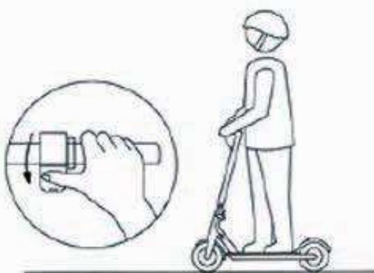
Gently pull the throttle trigger to begin picking up speed .
