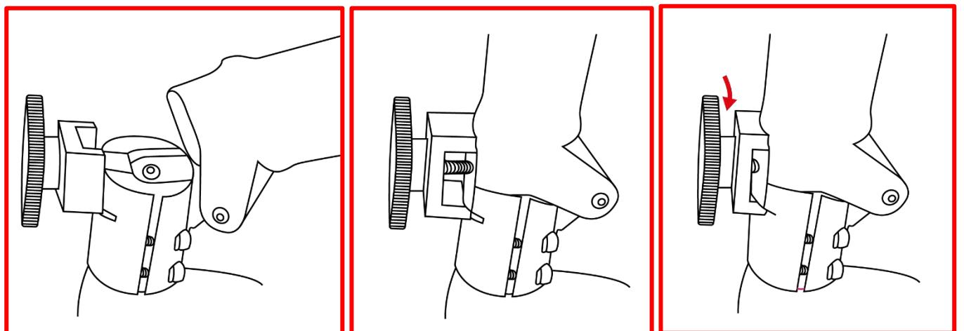
To unfold your scooter, straighten your stem vertically to the end. Once straightened, check the buckle to lock your scooter.
