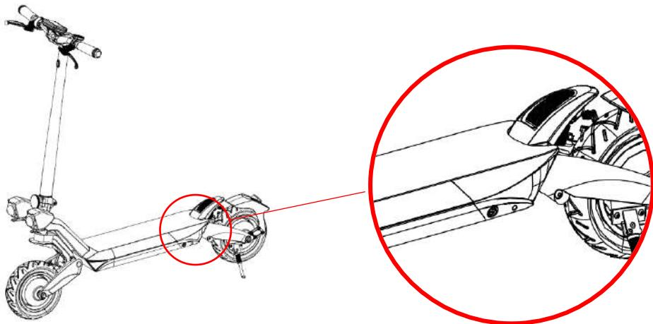
When charging your scooter, make sure the charging port is in good condition and that no residue is stuck in it. If it is, clean it with a dry cloth. Use the charger supplied with the product, and only that charger. If you have lost your charger, or it is defective, contact Urbanglide support. Once the charger shows a green light, unplug your product. Do not leave the charger plugged in for too long after charging is complete.
