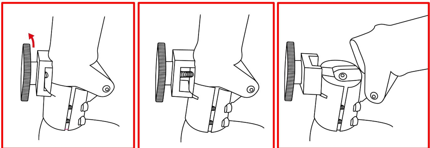
To fold your scooter, unscrew the buckle until the stem is free. Once released, lower the stem to fold your scooter. Lower your handlebars to the bottom to lock the folding.
