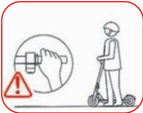
Do not press the accelerator when you are not on the scooter
