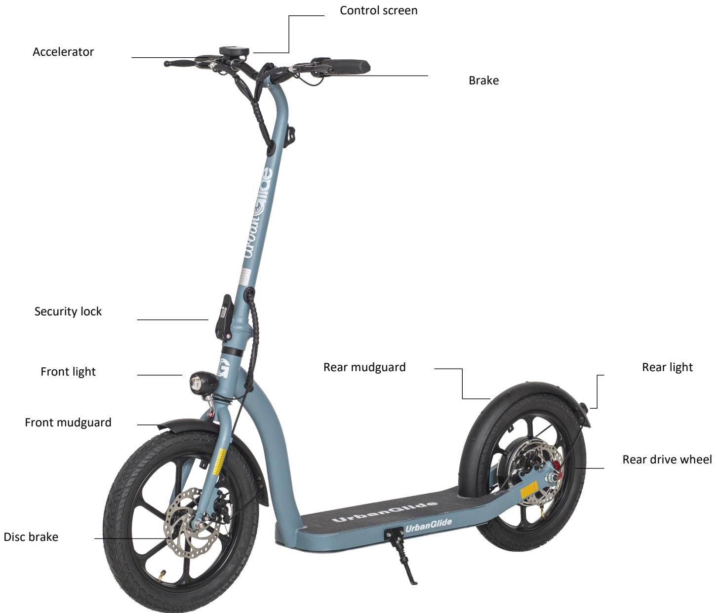
To move forward, turn on the scooter by pressing the button , start with speed 1 to apprehend the speed, to change gears press the button , place one of the two feet on the tray, give an impulse with your foot and use the right trigger on your handlebars to move your scooter forward. To turn on the light press the up arrow.
