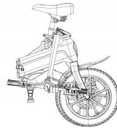
1. Open the handlebar quick release, adjust the handlebar.
