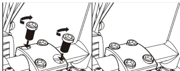
1 Use an M6 wrench, tighten bolts in a clockwise direction.
