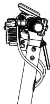
3. Insert the connector , and insert the T bar into the upright tube , then lock the screws on both sides .
